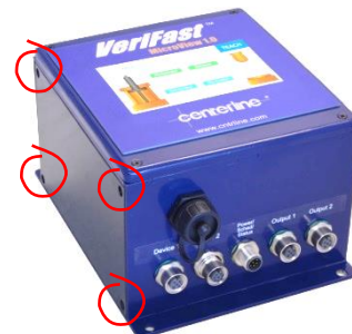
Figure 7 – Accessing the Signal Conditioner
